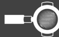
All of our machines are standardly equipped with 54mm-diameter portafilters. During coffee extraction, with the same incoming pressure, the 54mm weighs much less on the coffee puck compared to the classic 58mm. With the same amount of coffee, the 54mm ensures a taller coffee cake: hot water will take longer to flow through the coffee ground and with less pressure. The result will be a richer coffee, full-bodied and with complex aromas.
